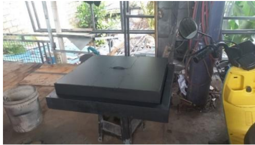
Gambar 5. Hasil pengelasan alas water shield
